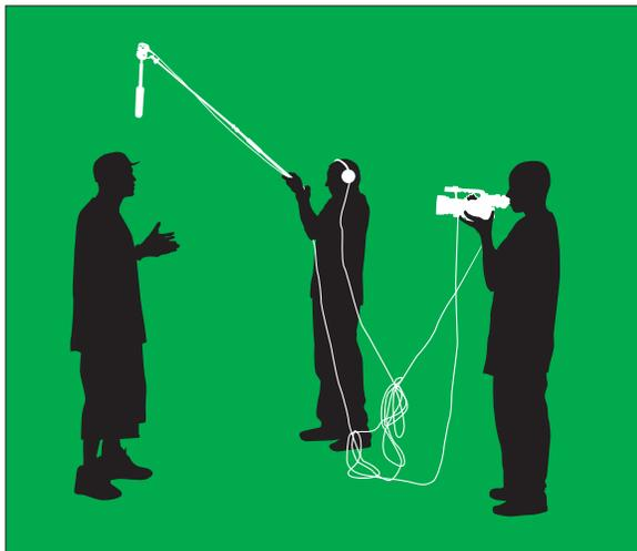
These microphones are mounted on a pole. They are designed to pick up sound only in the direction in which they are pointed and to minimize sounds at the sides and rear of the mic. Boom mics are ideal for isolating a subject's voice in a noisy or crowded environment.
